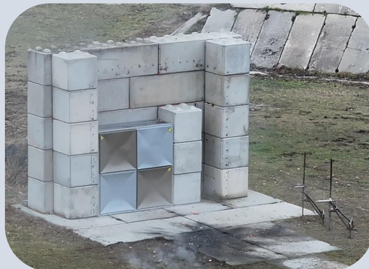
MEPS – lining after explosion of 3 kg TNT at a distance of 3 m
